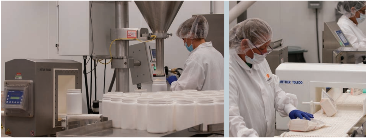
Using metal detection on filling lines and after packaging helps to keep the finished product contaminant free, reducing the risk of recalls
